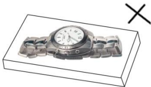
Never let the metal band touch the case back as it will effect the signal reception
